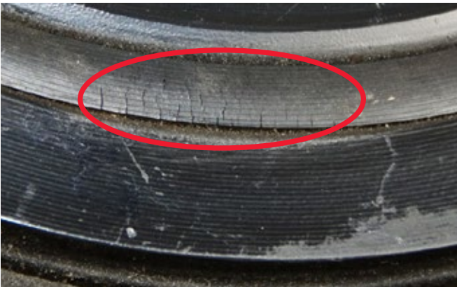
Cracked rubber on a stock rubber damper showing early signs of wear.
