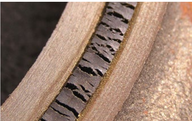
Stock rubber damper with advanced signs of wear.
