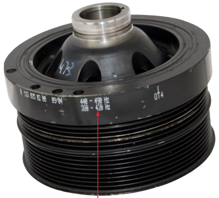
Elastomer or rubber harmonic balancers are tuned for a specific narrow frequency range.
